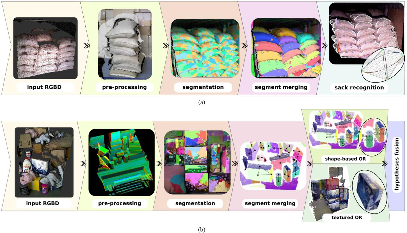
Fig. 4. The two instances of our perception pipeline, consisting of the respective processing steps from data acquisition to the hypotheses fusion. The pipeline for coffee sack perception shown in (a) relies on a single, dedicated object recognition module. In contrast, the pipeline for heterogenous goods perception in (b) fuses the results of a shape-based and a texture-based recognition module.
