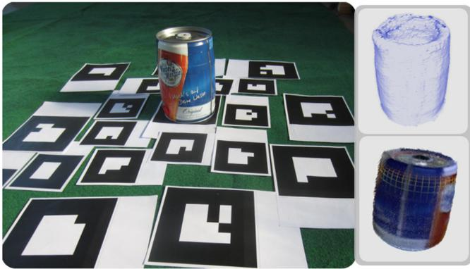
Fig. 5. Left: Database object acquisition setup. Right: Point-cloud and triangle mesh reconstructed models stored in the database.
