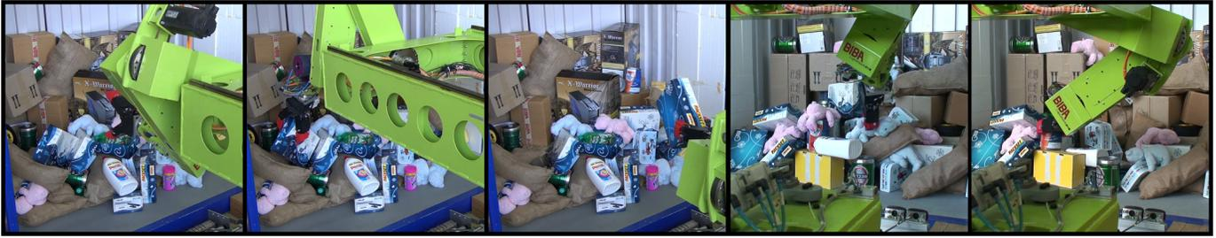
Fig. 9. Snapshots from an unloading sequence in a challenging cluttered scenario. Starting from a sensing pose, the robot approaches, grasps and extracts a parcel (frames one to three). Grasps acquired on a deformable teddy bear and a five liter barrel are shown in the next two frames.
