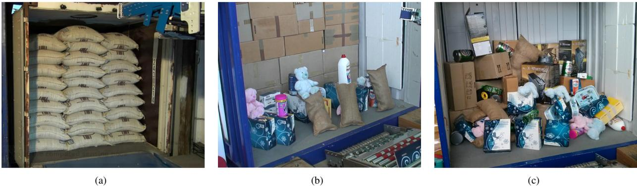
Fig. 7. Unloading of coffee sacks was evaluated on real-world scenarios at a warehouse owned by Vollers GmbH. A sample fully packed container is shown in Fig. 7(a). Unloading of loose goods was evaluated over many sample scenes (one instance shown in Fig. 7(b)). A more challenging cluttered evaluation scenario is shown in Fig. 7(c)
