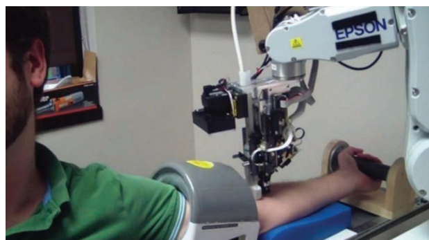
Figure 6. Automated blood taking using robotics. (Source: M. Yarmush, Rutgers University; used with permission.)
