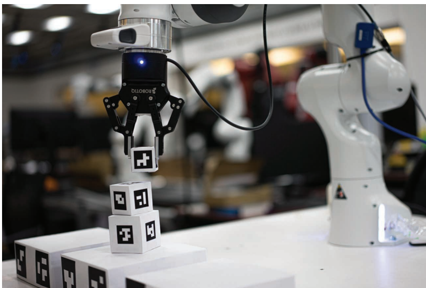
Figure 2. A robot using task and motion planning to solve the Tower of Hanoi puzzle. The robot consists of a Franka Panda arm and a Robotiq Gripper.
