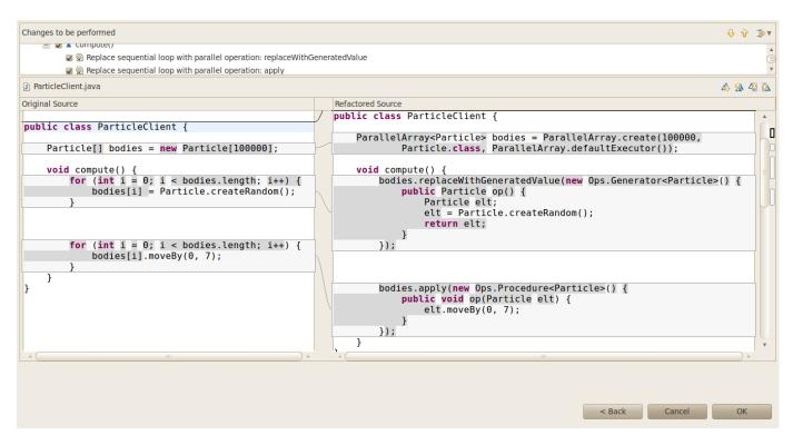
Fig. 2. Using a refactoring tool to parallelize loops using the ParallelArray library. The preview shows the sequential code on the left-hand side. The right-hand side shows all the changes that need to be applied.
