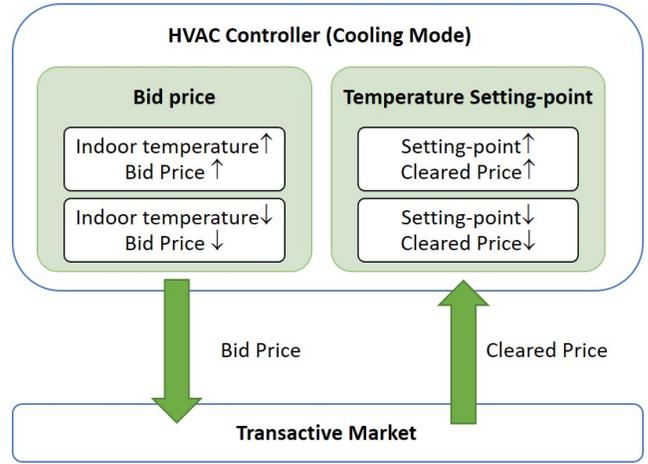
Fig. 4. Smart HVAC controller mechanism in cooling mode.
