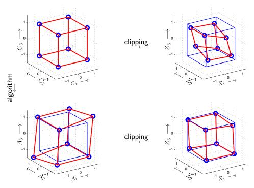
Fig. 6. Top row: visualization of the effect of clipping on the set of possible OFDM frames (here: N=3, 2-PAM per carrier). Bottom row: visualization of predistortion via an algorithm for maximizing the power of the signal after clipping.
