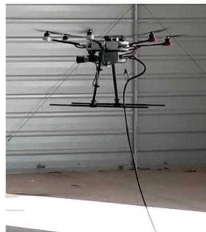
**FIGURE 1.** The captive drone used at SP Cup 2020 to capture all of the data sets, which were composed of the video and IMU data.
