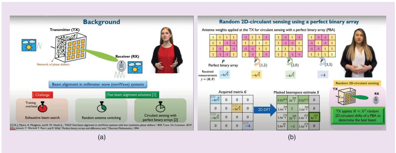
**FIGURE 2.** The video for fast beam alignment in mm-wave radios. (a) The background of the beam-alignment problem and (b) the random 2D-circulant sensing using a perfect binary array (PBA). Tx: transmitter; Rx: receiver; DFT: discrete Fourier transform.
