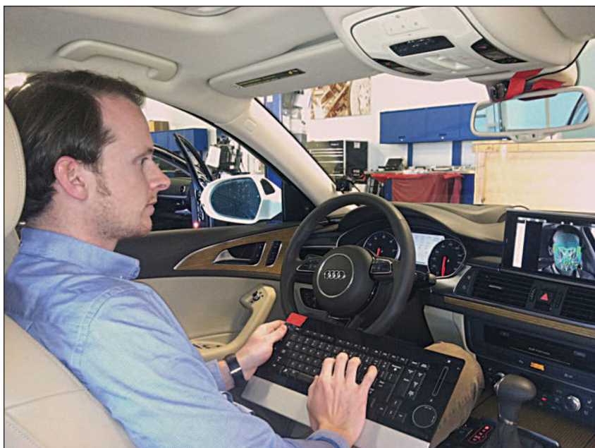
FIGURE 6 An engineer calibrates image-recognition software and its facial-mapping camera (mounted above the rearview mirror). Facial images are used in an app called Attention Guard to regain the driver's attention if he or she is not focused on driving [8]. (Figure courtesy of Audi AG, Ingolstadt, Germany.)
