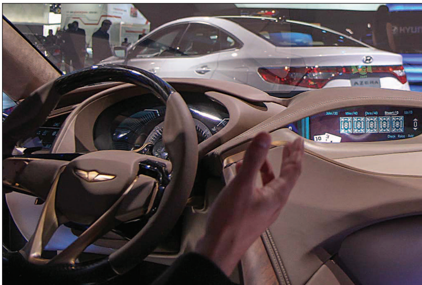
FIGURE 3 The Hyundai HCD-14 Genesis concept vehicle is shown without clusters of buttons and knobs. Instead, eye tracking and hand-gesture recognition systems are used to select and control specific features [5]. (Figure courtesy of Hyundai Motors USA, Fountain Valley, California.)
