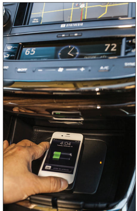
FIGURE 5 Toyota announced that its 2013 Avalon Limited will be the first vehicle to offer in-console wireless charging for Qi-enabled cell phones and devices [6]. (Figure courtesy of Toyota Motor Sales, Torrance, California.)
