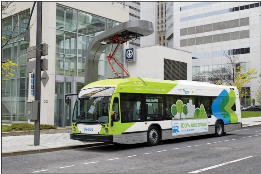
FIGURE 7 A fast-charging electric Volvo-Nova bus on STM Line 36-Monk [31]. (Source: STM; used with permission.)
