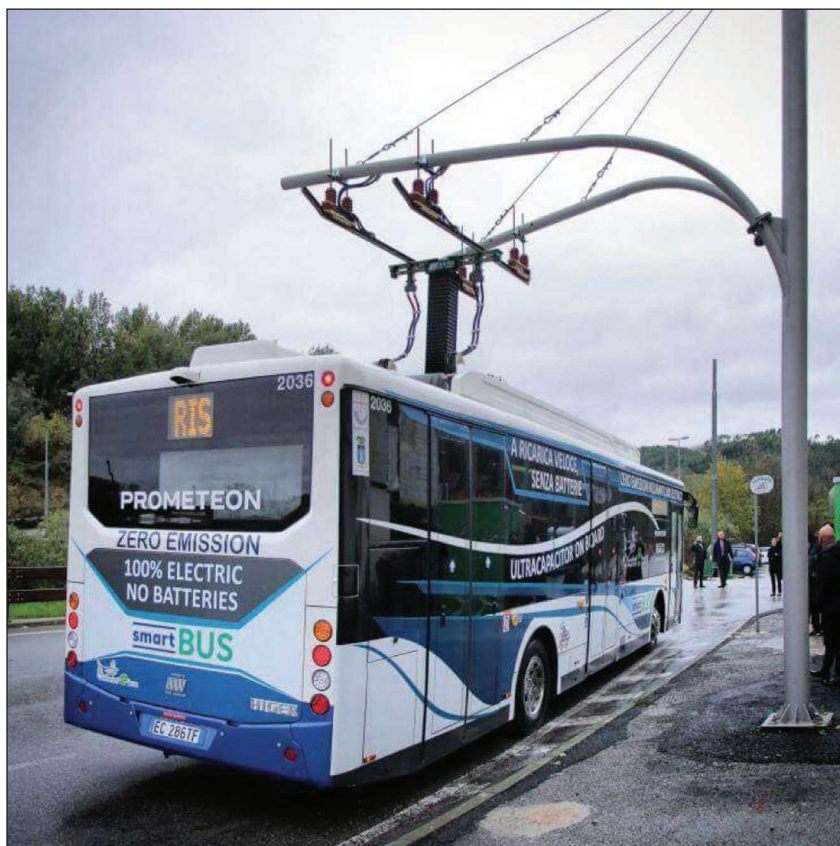
FIGURE 10 A Chariot Motors pure UC city e-bus and its fast charging system [11]. (Source: chariot-electricbus.com; used with permission.)
