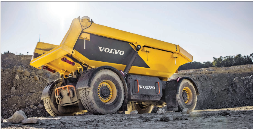
FIGURE 2 Volvo's autonomous and electrified hauler Tara.
