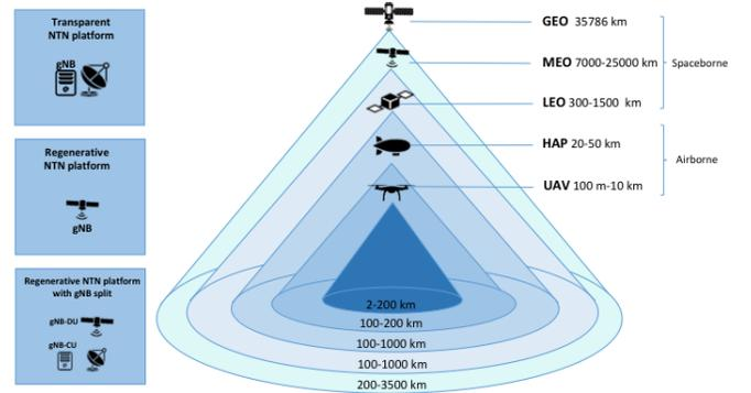
Fig. 3: NTN platform types and architecture options.
