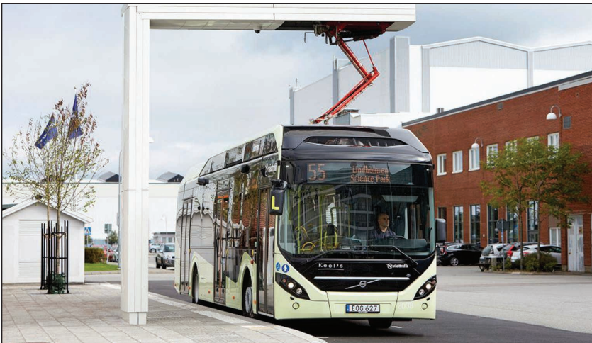
FIGURE 9 OppCharge electric bus charging station installed outside Volvo electric bus depot in Arendal, Norway. (Source: https://www.volvobuses.com/ , used with permission.)
