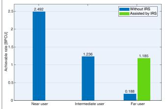
Fig. 4. Achievable rates when the SNR is 26 dBm for MIMO-NOMA and IRS-NOMA systems serving three users with fixed power allocation. The near user is located at 100 m, the intermediate user at 200 m, and the far user at 1500 m from the BS. The power coefficients for the near, intermediate, and far users are 1/10, 3/10 and 6/10, respectively.
