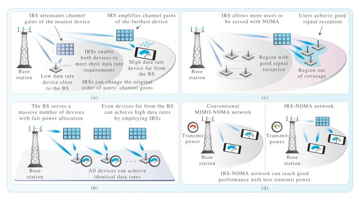
Fig. 1. Illustration of potential achievements of IRS-NOMA networks. (a) The IRSs can tune the channel gains to meet the data rate requirements of both near and far users. (b) The IRSs can boost the performance of the network under fair resource allocation. (c) By deploying an IRS at the cell-edge, more users can be served with NOMA. (d) The IRS-NOMA system can achieve similar rate performance of conventional MIMO-NOMA with less transmit power.
