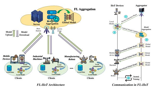
Fig. 1: The network architecture and communication process for FL-IIoT.
