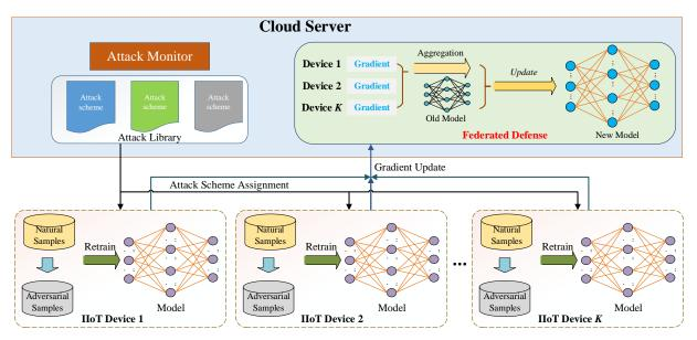
Fig. 2: Federated attack detection and defense in FL-based IIoT networks.
