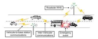
Figure 5: A very special WMN: The Vehicular Network. It consists of a set of cars and roadside WHSs that exchange messages to report some important events or offer services to the drivers.
