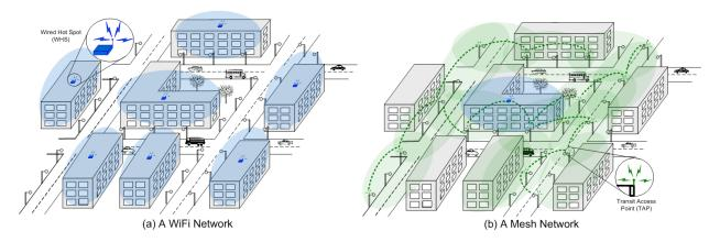
Figure 1: Two approaches to providing Internet connectivity. (a) WiFi Network: several Wireless Hot Spots (WHSs) are needed to offer good coverage of a given area; (b) Wireless Mesh Network (WMN): by using one WHS and several Transit Access Points (TAPs), it is possible to cover the same area as in (a); the TAPs rely on the WHS to transmit their traffic to and from the Internet.
