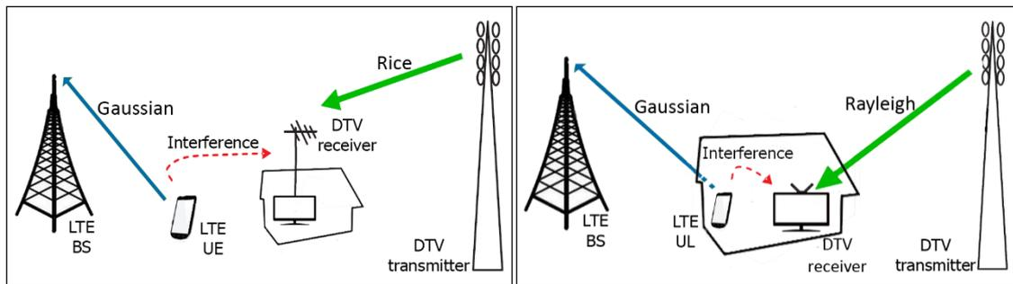
Fig. 1. Critical scenarios for LTE-UL interference: fixed (left) and indoor (right) DTT reception.
