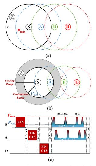
Fig. 2: (a) Ranges of nodes transmitting control signals using  $P_{max}$ ; (b) ranges of nodes after application of power control; (c) illustration of a uni-directional FD transmission at the MAC layer.
