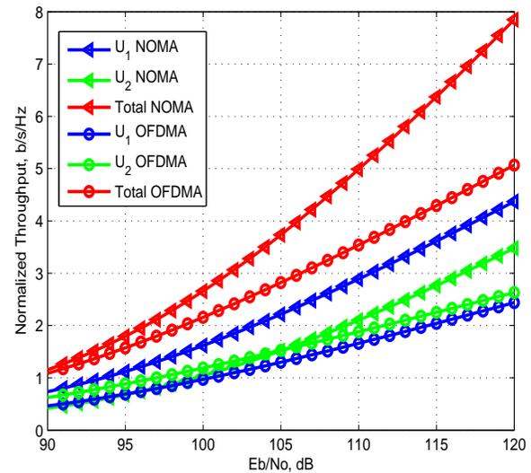
Fig. 4: Normalized System Throughput for Two Users
