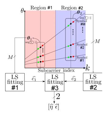
Fig. 1. The framework of the proposed technique.  $\theta$  denotes the extra phase rotation caused by CFO and SFO. Q = 2. The red dot and green dot form a pairwise correlation pair.
