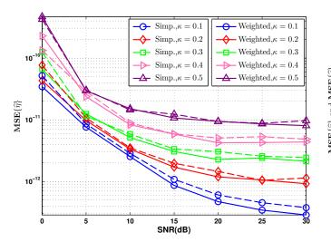
Fig. 6. MSE $\{\hat{\eta}\}$  under different accuracy of channel estimation;  $\kappa \in [0.1: \text{Fig. 7.} MSE\{\hat{\eta}\}$  and MSE $\{\hat{\epsilon}\}$  under different terminal velocity;  $M = \{0, 1\}$ 0.5],  $M = 10, Q = 4, \eta = 5 \times 10^{-5}, \epsilon = 0.02$ , and SNR  $\in [0, 30]$  dB.
