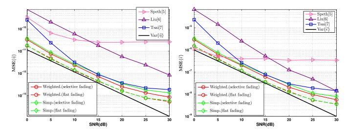
Fig. 2.  $MSE\{\hat{\eta}\}$  comparison among different estimators; M = 10, Q = Fig. 3.  $MSE\{\hat{\epsilon}\}$  comparison among different estimators;  $M = 10, Q = 4, \eta = 5 \times 10^{-5}, \epsilon = 0.02$ , and  $SNR \in [0, 30]$  dB.  $4, \eta = 5 \times 10^{-5}, \epsilon = 0.02$ , and  $SNR \in [0, 30]$  dB.
