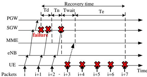
Fig. 5: Timing diagram of 3GPP recovery mechanism.
