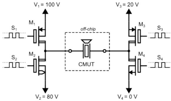
Fig. 2. Schematic of the differential output stage. Note that  $M_2$  is an isolated NMOS located in its own well.
