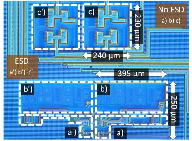
Fig. 5. Picture of the taped-out differential transmitting circuit.
