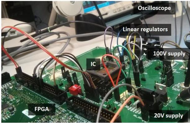
Fig. 6. Setup for the integrated circuit measurements.
