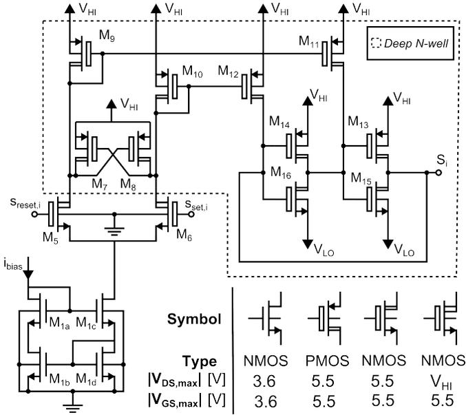
Fig. 3. Schematic of the improved level shifters.
