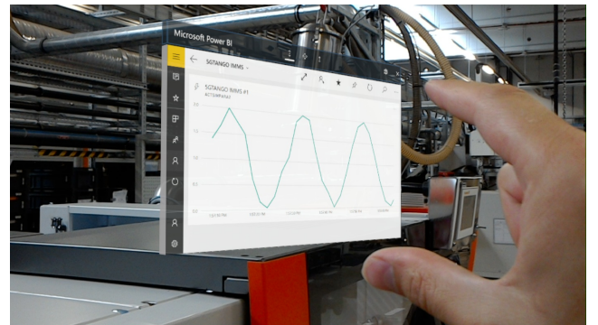
Fig. 2: Demonstration of using Microsoft Power BI for data visualization on Microsoft HoloLens
