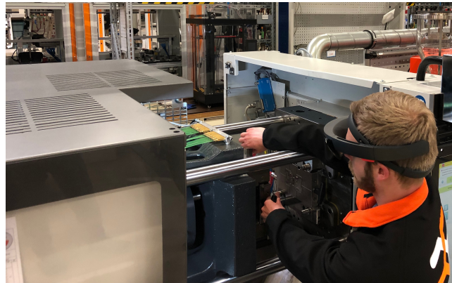
Fig. 1: Application of Microsoft HoloLens for remote maintenance of an injection molding machine's tool
