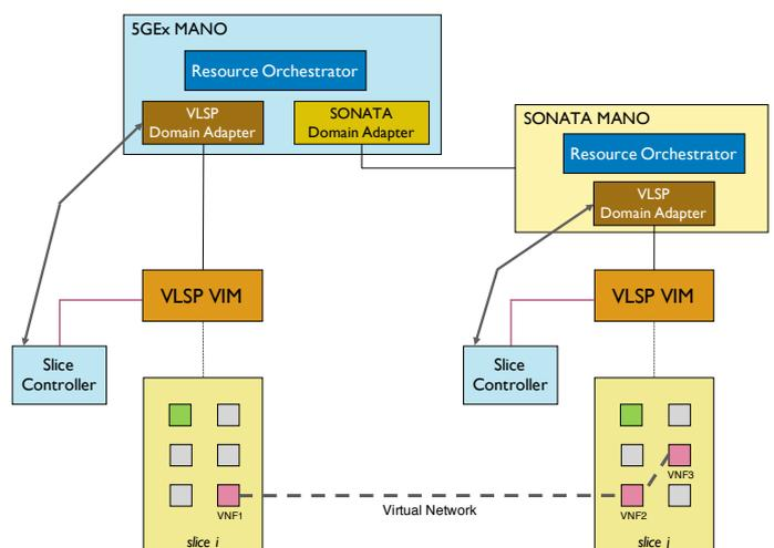
Fig. 5. Multi-MANO setup on a sliceable NFVI
