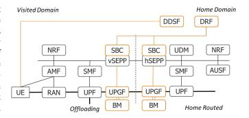
Fig. 3. Extended Inter-NPN Roaming Architecture
