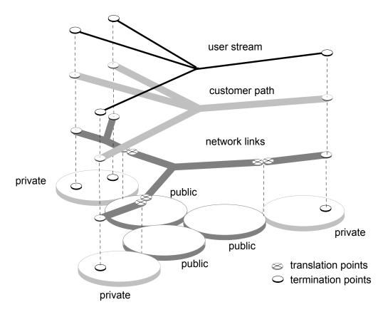
This figure shows the core structural concepts identified in the information viewpoint of the VPN design and how they map onto the different types of network domains involved.
