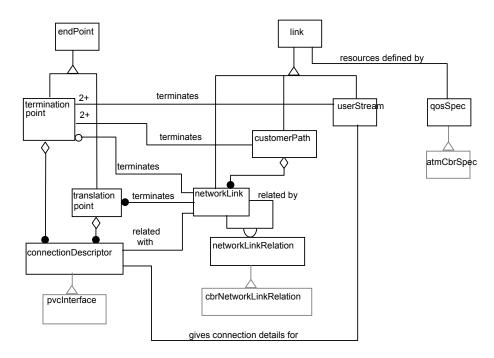
The figure above shows the overall information model for the VPN service expressed in OMT notation. The core concepts of customer path, network links, user streams, termination points and translation points have all been mapped straight onto this information model.
