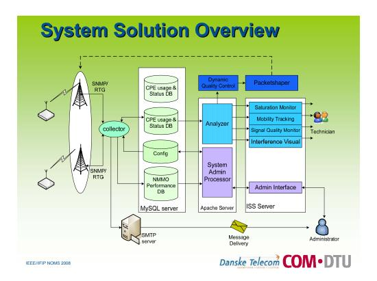
WiMAX network monitoring and optimization system can be divided into six main function blocks:
