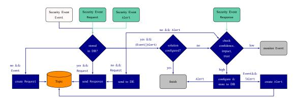
Fig. 2: Data flow of the communication process within MiR from the perspective of one ISP
