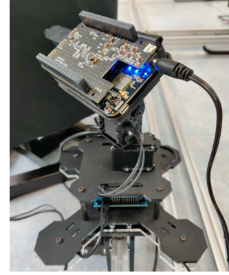
FIGURE 25. PhantomX Robot Turret [30] with mounted RX front-end, used to adapt the RX orientation.
