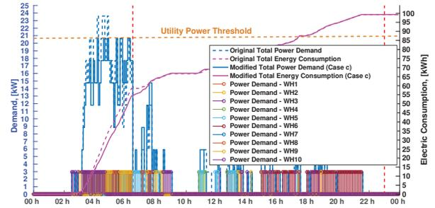
Fig. 4: Case (c). Peak shaving by purely switching the houses to the energy model.
