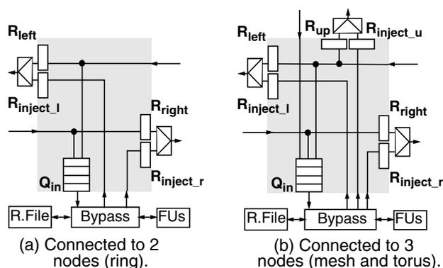
**Figure 3. Router schemes for asynchronous point-to-point interconnects**
