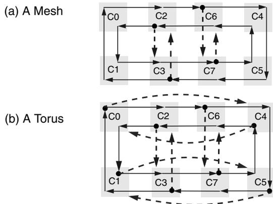
**Figure 5. Additional topologies for 8 clusters. A black dot at the end of a link means that there is more than one link that can be followed for the next hop if the corresponding node is not the destination. Messages can always be routed through solid links but dashed links represent the end of the corresponding path; thus, they are only used when they are the final ones.**
