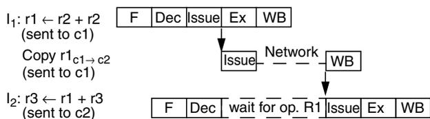
**Figure 2. Sample timing of a communication between two dependent instructions  $I_1$  and  $I_2$ , steered to clusters  $c1$  and  $c2$  respectively (the arrows mean wakeup signals, and communication latency is 2 cycles).**
