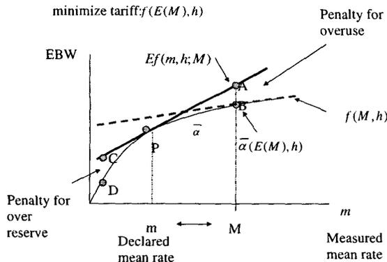
Figure 3.1 Effective bandwidth versus mean rate  $m$  under fixed peak rate  $p$ , capacity  $C$ , and buffer  $B$ .
