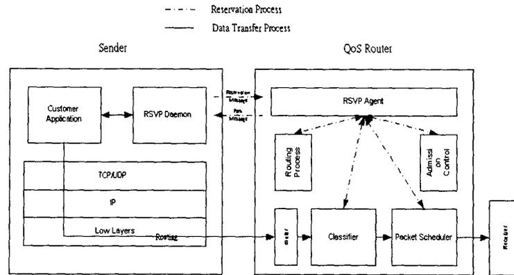
Fig 2.1 An router architecture for guaranteed QoS service
