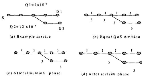
Fig 2.2 An example of allocation and reclaim phase
