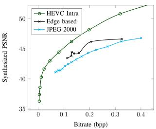
Fig. 4: Rate-Distortion performance of synthesized  $V_4$  with the bitrate of  $V_3$  depth map, for different quality factors of JPEG2000 and HEVC, and different Sobel detection thresholds of our method.
