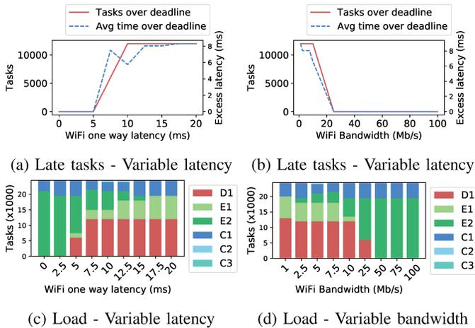
Fig. 10: Impact of WiFi latency and bandwidth on task allocation and excess latency. For latencies  $> 5$  ms, in-time completion rate drops to 50%. Minimum completion rate is achieved for bandwidth  $> 25$  Mb/s
