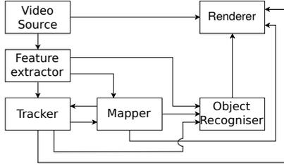
Fig. 1: Main components of a typical MAR application.
