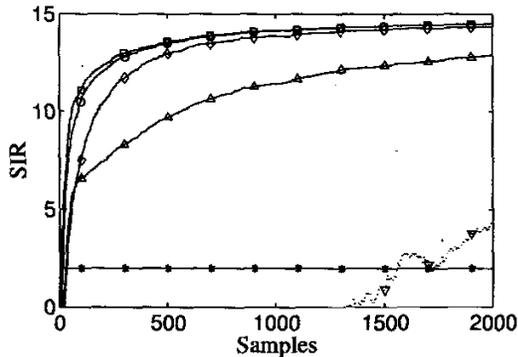
Fig. 1. Convergence for MMSE ( $\circ$ ), BH ( $\square$ ), WWH ( $\diamond$ ), HWW ( $\Delta$ ), MF ( $*$ ) and PASTd ( $\nabla$ ) for synchronous CDMA with  $n = 8$  users, MAI=30dB and SNR=15dB.
