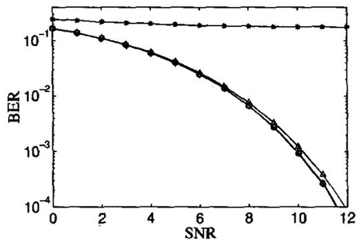
Fig. 2. Bit Error Rate for MMSE ( $\circ$ ), BH ( $\square$ ), WWH ( $\diamond$ ), HWW ( $\Delta$ ), MF ( $*$ ) for synchronous CDMA with  $n = 8$  users and MAI=30dB.
