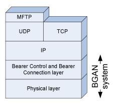
Figure 1 Operation of MFTP over BGAN system
