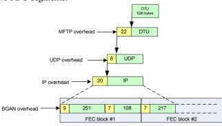
Figure 4 Data Transfer Mapping between MFTP over BGAN
