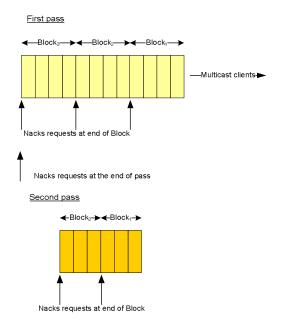
Figure 2 MFTP Pass, MTFP Block and Data Transfer Unit
