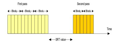
Figure 3 Status Retry Timer in MFTP
