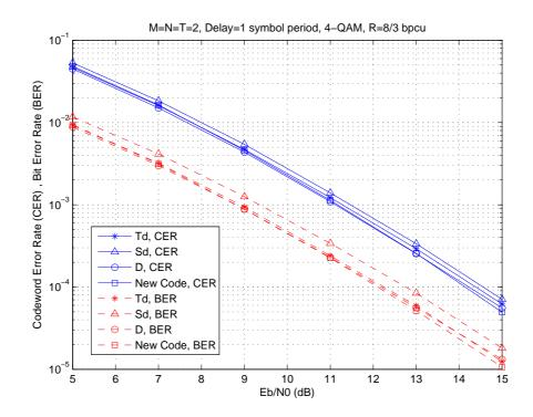
Fig. 6. Performances of the codes  $\Gamma$ , D, T<sub>d</sub> and S<sub>d</sub> with a delay of 1 symbol period
