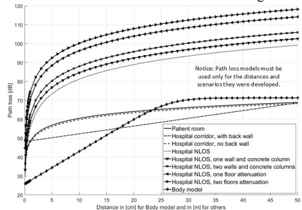
Figure 3. Path loss values as a function of distance.
