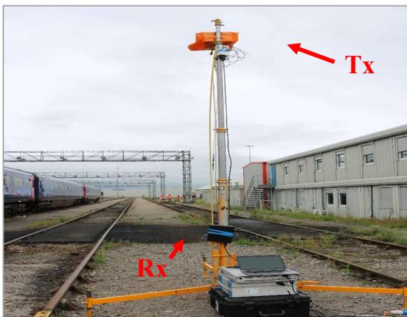
Fig. 1. 60 GHz transmitter setup using Keysight M8190 AWG and Siverts IMA, and the measurement scenario.
