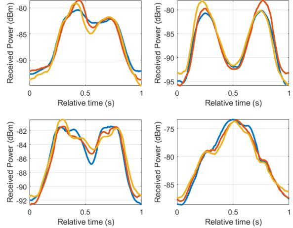
Fig. 2. Gait cycles plotted on top of each other. The received power is similar for the same user, but different between users.
