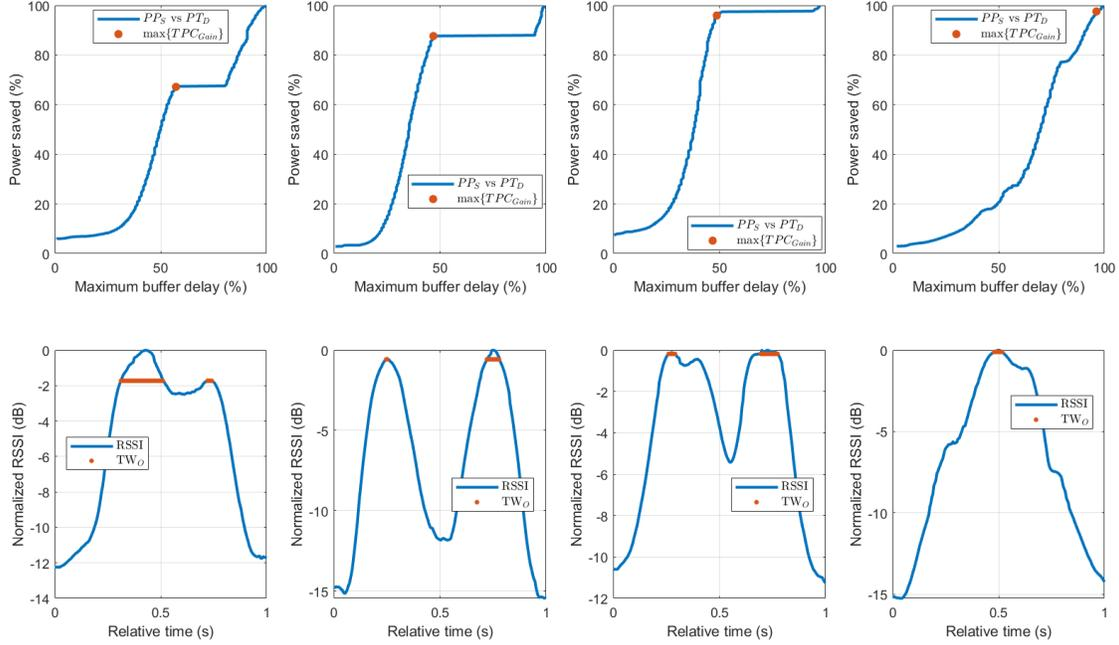
Fig. 3. Top row, the relationship between percentage power saved and percentage maximum buffer delay for different gait. The point of  $\max\{TPCGain\}$  is indicated by a red dot. Bottom row, the RSSI values for the corresponding gait. The optimal transmission window  $TW_O$  is indicated by red dots.
