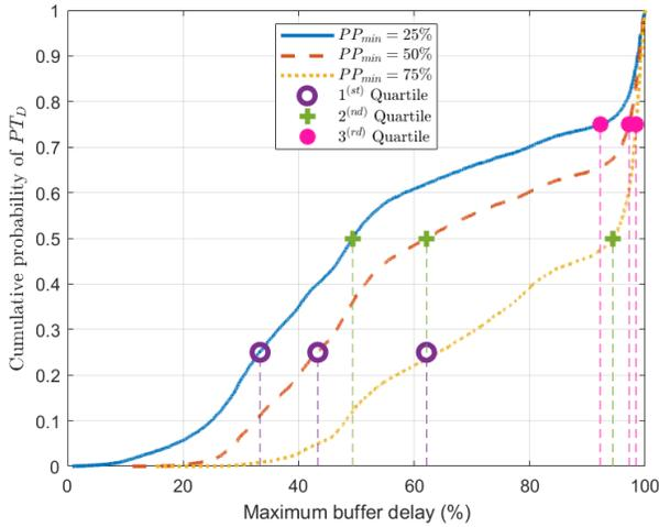
Fig. 5. Cumulative probability of maximum buffer delay  $PT_D$  for the optimal transmission window  $TW_O$  where the minimum power saving requirement  $PP_{min}$  is set to 25%, 50%, and 75%.
