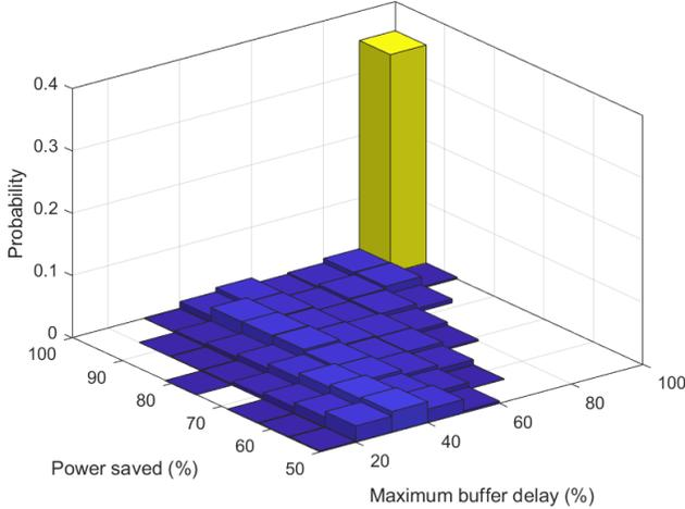
Fig. 4. The probability distribution of power saved  $PP_S$  and maximum buffer delay  $PT_D$  for the optimal transmission window  $TW_O$  where the minimum power saving requirement  $PP_{min}$  is set to 50%.
