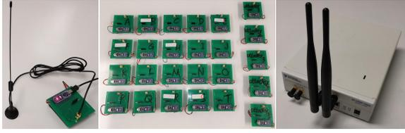
Fig. 1. Devices used in the experiments. Left: a DUT in operation. Middle: 20 DUTs as legitimate devices and 5 DUTs as rogue devices. Right: a USRP-2922 platform as the receiver.
