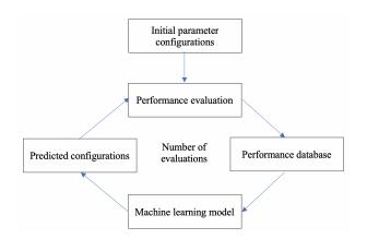
Figure 1. Machine-learning-based autotuner ytopt
