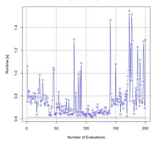
Figure 5. Autotuning syr2k using ET in 200 evaluations
