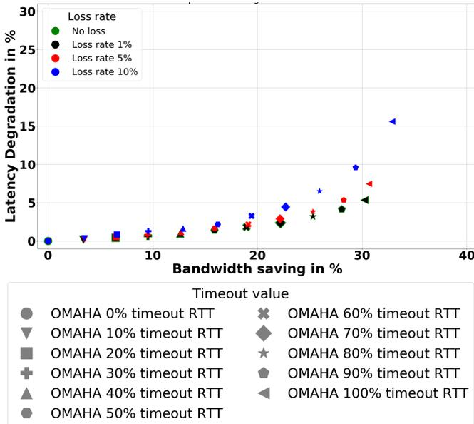
Fig. 6. Impact of messages loss on Paxos
