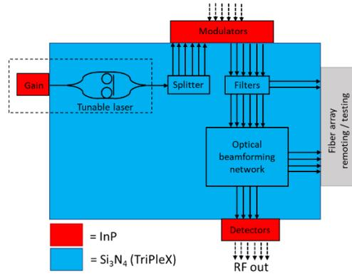
Fig. 1. Block diagram of an integrated optical beamformer
