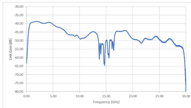
Fig. 3. Measured link gain of the integrated optical 1x4 beamformer.
