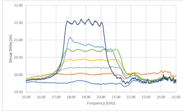
Fig. 4. Measured delay applied by the integrated optical 1x4 beamformer.
