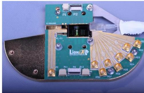
Fig. 2. Photograph of an state-of-the-art of an integrated optical 1x4 beamformer module.
