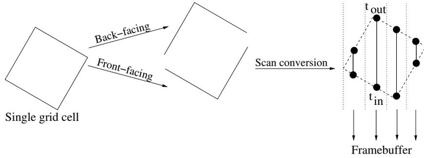
Figure 2: Cell-projection process.
