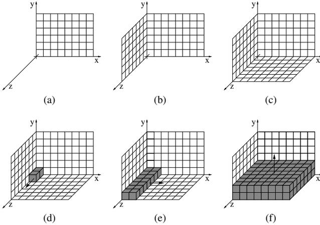
Figure 3: Rendering order of grid cells — all components of  $\vec{r}\vec{v}$  (the vector pointing toward the viewer, see Figure 4(a)) being positive. First, all back-facing faces of the first layer of cells in each direction are rendered (a) – (c). Second, all cells are rendered. The order in which axes are handled (first- $z$ —then- $x$ —then- $y$  order) is arbitrary. Only the order according to which cells are handled along an axis is important.
