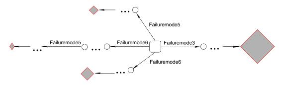
Figure 7. A portion of the counterexample visualisation in the case of  $\mu$ C, FET and FASIC failures
