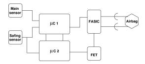
Figure 1. Schematic system architecture
