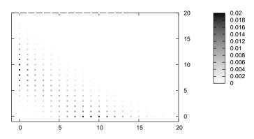
Fig. 3. Exclusive switch at time 10000. The x-axis gives the number of  $N_1$  molecules and the y-axis gives the number of  $N_2$  molecules. Each point of the plot corresponds to the states of systems that have the have the corresponding number of  $N_1$  and  $N_2$  molecules. The darker the point is, the more probability mass it holds. We can notice the bistable behaviour from the two regions of black points, one for  $N_1 = 0$  and one for  $N_2 = 0$ .
