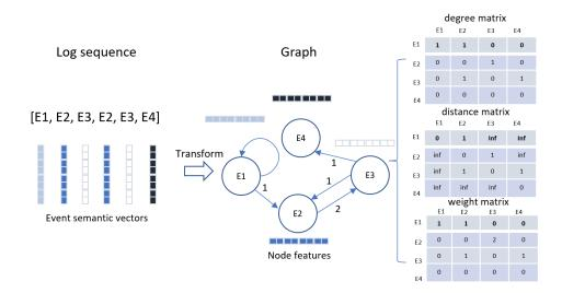
Figure 3. The diagram of the graph construction from a log sequence.
