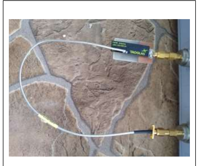
Fig. 5. The fabricated Meander antenna
